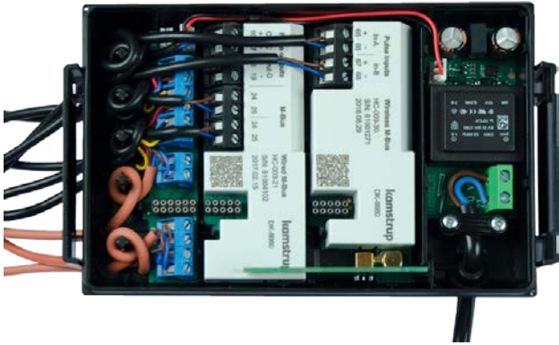
Wireless M-Bus module with internal antenna
